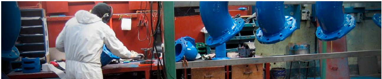
FIG. 1 Plascoat PPA 571 coating process
